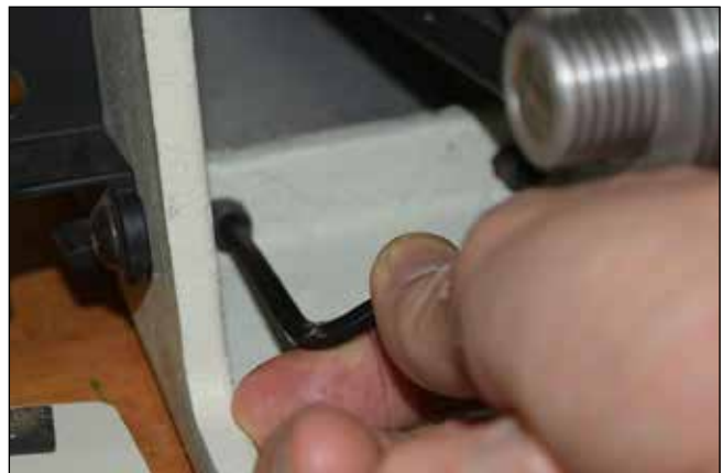
5 - Check that all bolts connecting the headstock to the lathe ways are tight.
