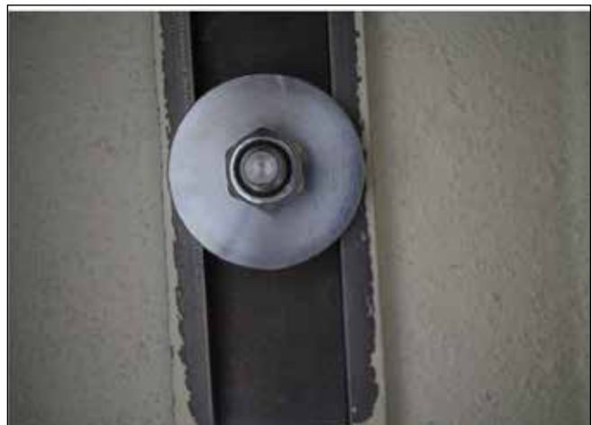
6 - Movable headstocks must be securely locked to the ways. Check the locking plate beneath the ways.
