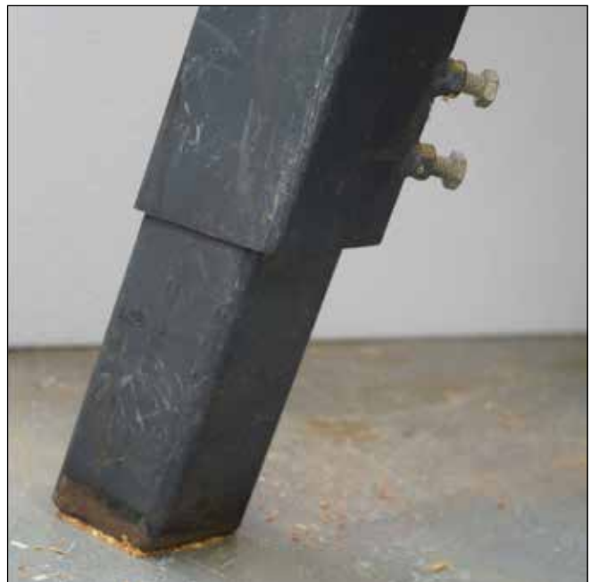
1 - Adjust legs, or use shims, to make sure your stand sits solidly on the floor.
