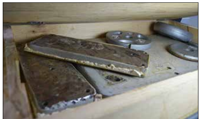
3 - Additional weight helps a lathe absorb vibration. Use steel plate, barbell sets, or sandbags
