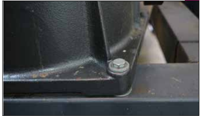
4 - A washer was inserted between the lathe and the stand to fill the gap, before tightening the mounting bolt.
