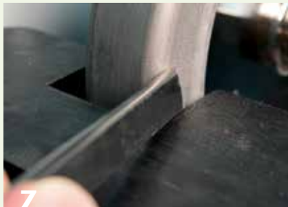
6 CBN wheels come in a range of grits and configurations. Some have a side flange that allows for sharpening on the side of the wheel—something you should never do with a friable wheel.
