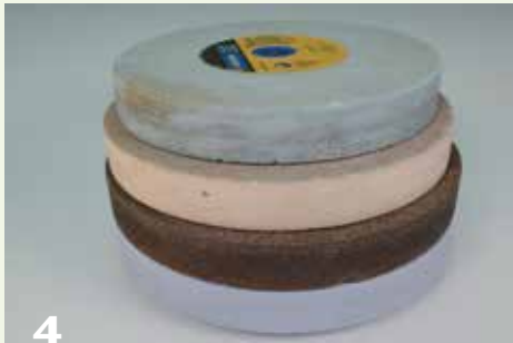
4 Colors are one indication of a wheel's material and coarseness. All of these friable wheels started at 8" diameter, showing that they wear away with use.
