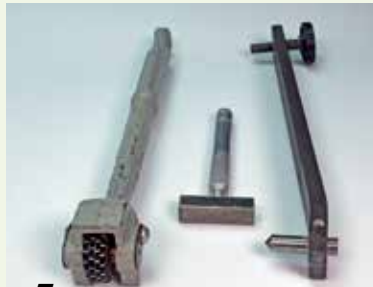
5 Friable wheels require supporting accessories to keep them in good shape. These tools are used to expose fresh grit, remove any unwanted grooves, and to true up the wheel.
