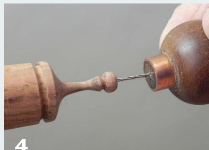
4 Pre-drill for the eye screw, using the indentation from the tailstock live center to help position the drill bit.
