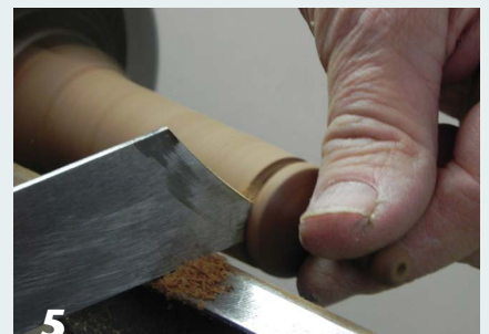
5 Undercut the top finial as it is parted off by angling the point of the tool to the right.
