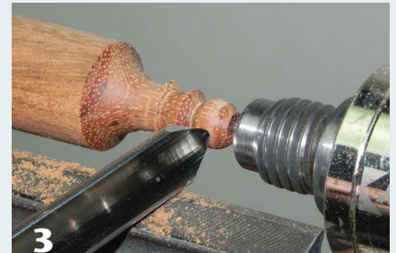
2 A peeling cut is one way to form the tenon.
