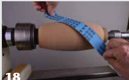
18 Hold a strip of sandpaper diagonally against the form to smooth out high spots. Note that the toolrest has been moved out of the way.
