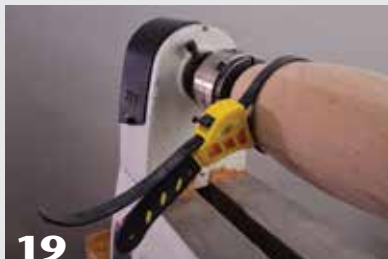
19 A strap wrench is invaluable in gripping the completed vase when removing it from the screw chuck.
