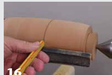
16 Mark the curve change point on the vase, then turn it to your desired shape.
