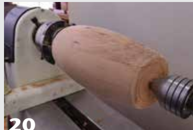
20 Mount the scrap jam chuck turned earlier in the scroll chuck. Then reverse-mount the vase, positioning the hole in the top on the jam chuck. Tailstock pressure holds the work in place as you complete the bottom.
