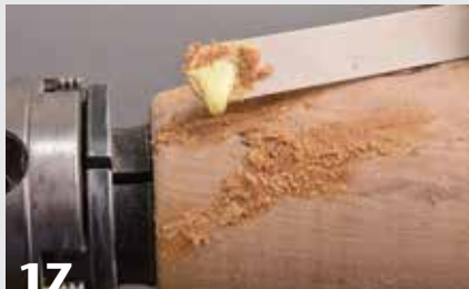
17 Fill any gaps in the glue joints with a paste of sanding dust and yellow glue.
