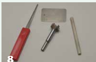
A diamond hone, a card sharpener, and a ceramic hone are examples of the few simple tools needed to keep Forstner bits sharp and cutting cleanly.
