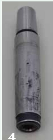
(4) Closely inspect, clean, and dress the drill chuck arbor.
