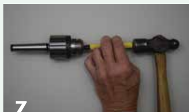
A drill chuck arbor separates from the head with a punch and sharp hammer tap for easy replacement.
